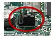
PONTECH Quick-240: Similar to the UAV except rotated and you short the two pins next to the jumper instead of using a button
